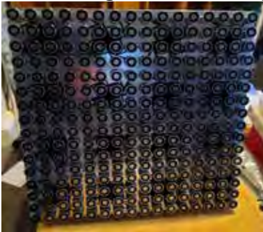
Figure 2.3.5 - FLEXeMAG end-effector showing the array of individually addressable electromagnets
