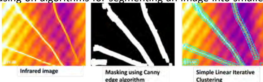
Figure 2.4.6 - (L) Infrared image of heated wires (C) Masked image using Canny edge detection algorithm (R) Image obtained using Simple Linear Iterative Clustering
