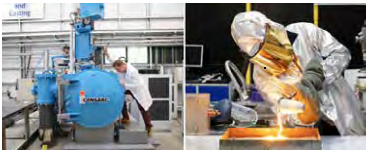
Vacuum induction melting for production of bespoke steel compositions of 4.5 – 7 kg ingot size (left) and casting of small (approximately 1 kg) ingots in air (right).
