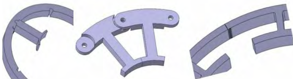
Figure 1.1.4: left; tapered tooth, middle; hinged structure, right; engineered core-back joint initial work shows that the position and tolerance of the module joints influence machine performance; especially cogging torque and the magnitude and harmonic content of the back EMF.
