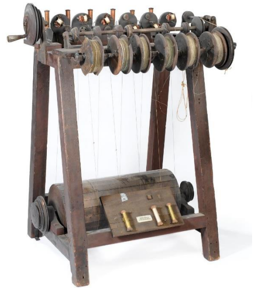
Figure 1: Science Museum Group. Machine used for covering wires with silk and cotton, 1837. 1939-139 Science Museum Group Collection Online, https://collection.sciencemuseumgroup.org.uk/objects/co44548/machine-used-for-covering-wires-with-silk-and-cotton-1837-winding-machine
