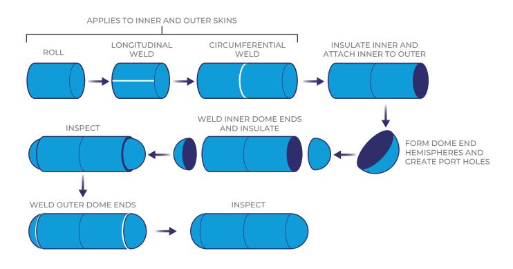
Figure 9 – Example manufacturing flow for a double-walled and insulated metallic tank
