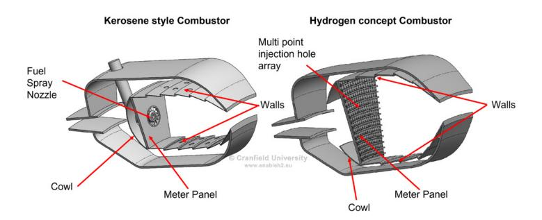
Figure 14 – Comparison of kerosene style combustor (left) and hydrogen concept combustor (right) from ENABLEH2 project. Image © Cranfield University
