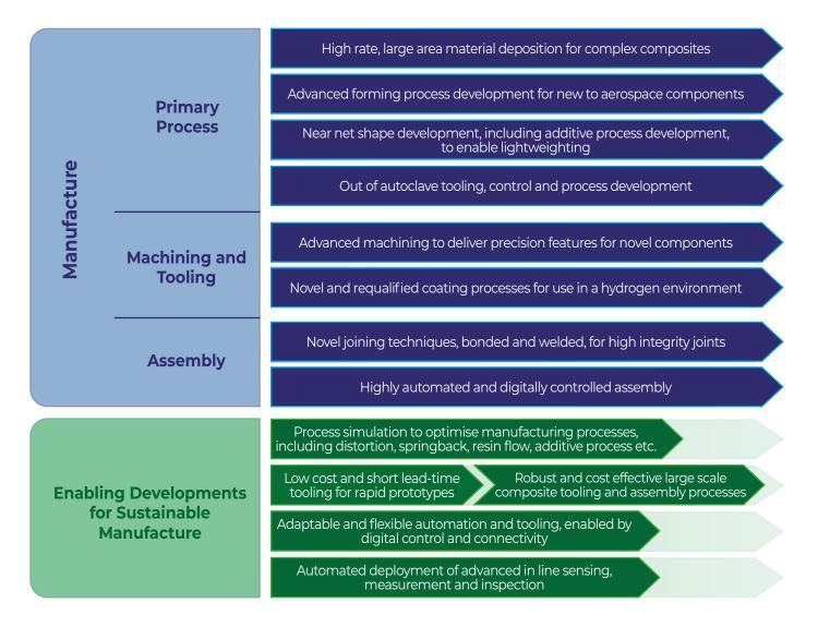
Figure 2 – Areas of manufacturing technology development identified in this paper are required to support the FlyZero technology bricks
