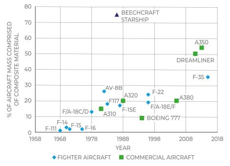
Figure 12 – Composite use in airframes. Adapted from **[35]**, with addition of data point for A350
