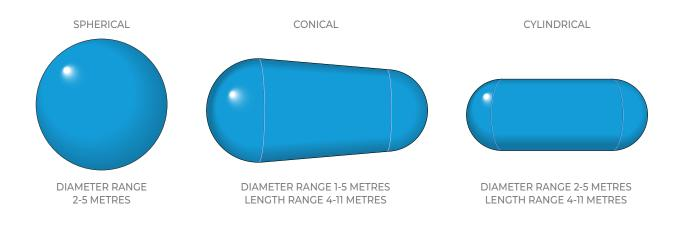
Figure 7 – Potential shapes and expected size ranges for liquid hydrogen tanks, from FlyZero concepts
