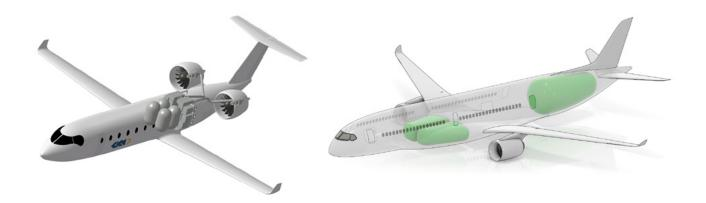
Figure 4 – Concept hydrogen aircraft. Left: liquid hydrogen fuel cell electric concept for a sub-regional aircraft from the GKN H2GEAR project (image © GKN). Right: FlyZero midsize concept FZM-1E with liquid hydrogen fuel tanks highlighted in green. Two tanks are located in 'cheeks' to manage the centre of gravity.
