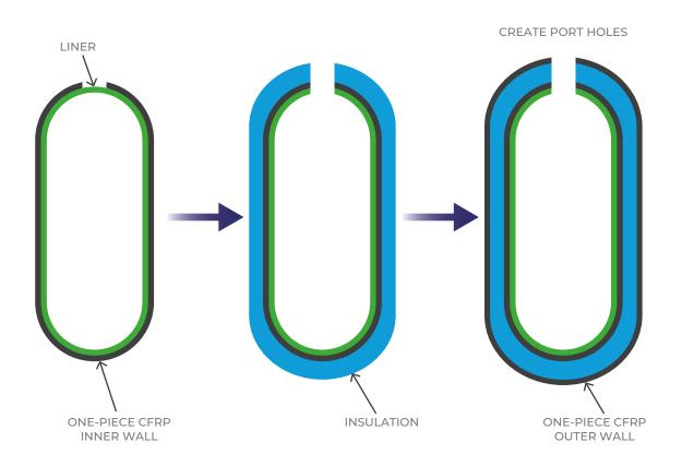
Figure 11 – Illustration of possible manufacturing process flows for double-walled polymer composite tanks
